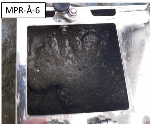
Figure 4-2: Photos of samples from MPR-Å-1 and MPR-Å-4 – MPR-Å-6, representing the seabed sediments in the investigated area. The sediments in MPR-Å-1 in Leirpollen 1 had a light grey colour and had more coarse grained material than the sediments in Leirpollen 2. The sediments in MPR-Å-4 had a high content of organic material. MPR-Å-5 contained parts of broken shells in addition to sand and gravel. The sediments in MPR-Å-6 consisted of mainly fine sand.
