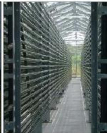
Fig. 3 A high-end closed bioreactor system. The worlds largest closed photo-bioreactor in Klötze, near Wolfsburg, Germany (Bioprodukte Prof. Steinberg; www.algamed.de ); the 700 m 3 are distributed in 500 km of tubes and produce up to 100 t algae biomass per year
