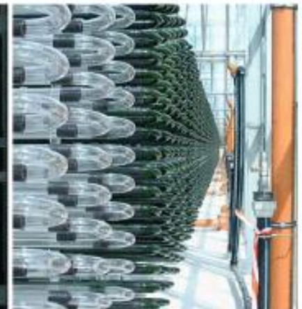
Fig. 3 A high-end closed bioreactor system. The worlds largest closed photo-bioreactor in Klötze, near Wolfsburg, Germany (Bioprodukte Prof. Steinberg; www.algamed.de ); the 700 m 3 are distributed in 500 km of tubes and produce up to 100 t algae biomass per year
