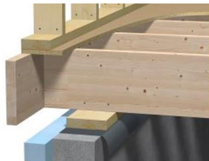
Splitta limtre (S-bjelke, Splitkon )
